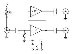
Figure 55-3 PA-300 Preamp Equivalent Circuit
