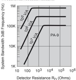
Gain/Bandwidth Specifications Model PA-9 Preamplifier
