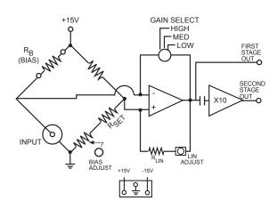
Figure 55-4 PA-8200 Preamp Equivalent Circuit
