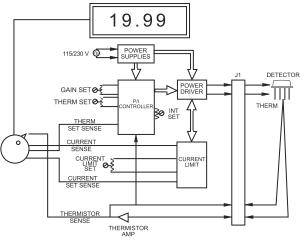
Figure 1 TC5 Block Diagram
