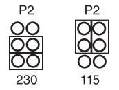
4. To change the AC configuration, remover the jumpers and place them according to the diagram above.
