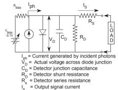
Output signal current from detector I<sub>s</sub> is defined as:
