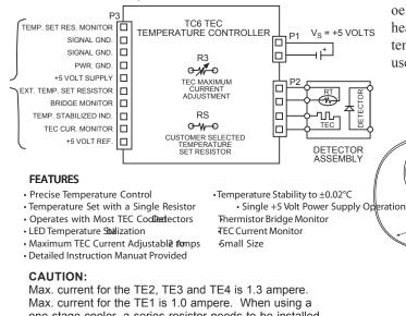
one stage cooler, a series resistor needs to be installed with the TC to limit the max. current to 1.0 ampere.
