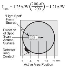
Series resistance is approx. 0 at contact. Total series resistance is approx. 5 - 10 , approx. 6 nominal. Therefore, response uniformity is a function of the voltage divider in the equivalent circuit  $R_{\rm D}$  and  $R_{\rm S}$ .
