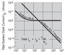
Detector Shunt Resistance R<sub>D</sub> (Ohms)
