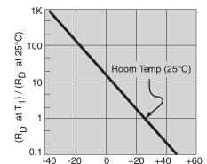
Change in Shunt Resistance vs Temperature
