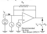
$\rm Max.~R_{_{\rm F}}$  for InSb determined by (I $_{\rm BG}$ ) Fig. 19-5. Max. recommended DC voltage is 5 volts. V offset =  $I_{BG} \times R_{F}$
