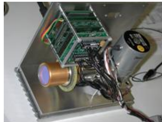
J508 with RICOR micro-cooler (LN 2 )
