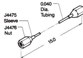
J9181 Tubing and Fitting Assembly (single end)
