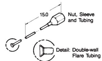
Assembly of Nut, Sleeve and Tubing with J5121 Adapter (optional)
