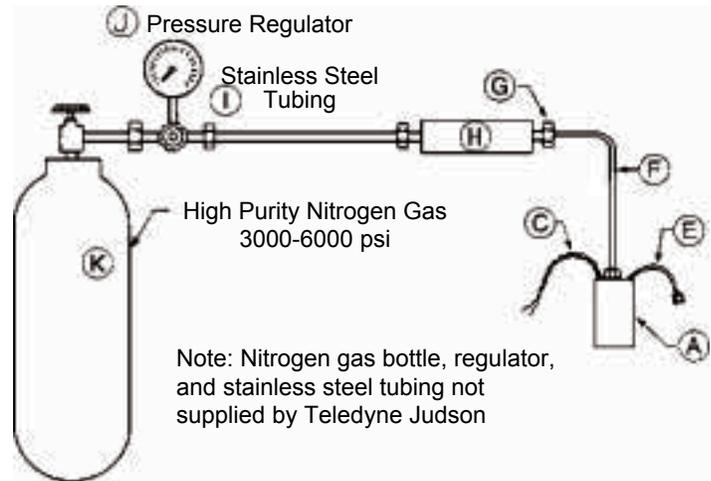
Figure 3: Suggested operating setup for the JTC system
