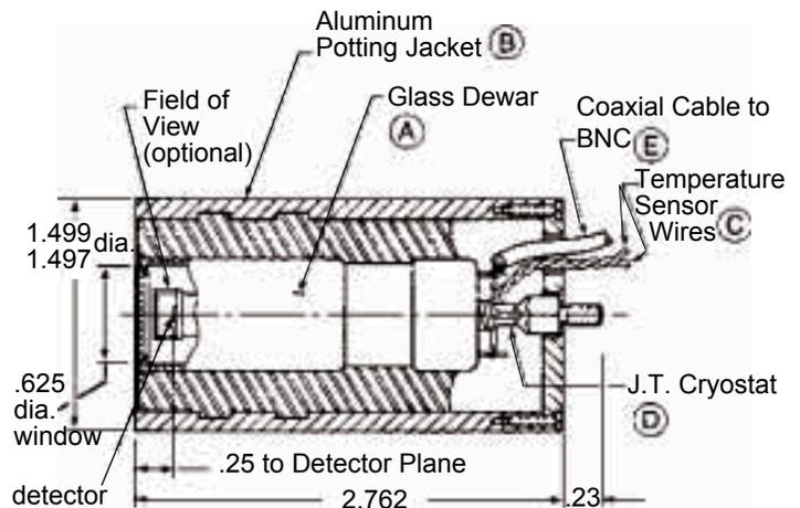
Figure 4: Detector/Dewar/Cryostat assembly
