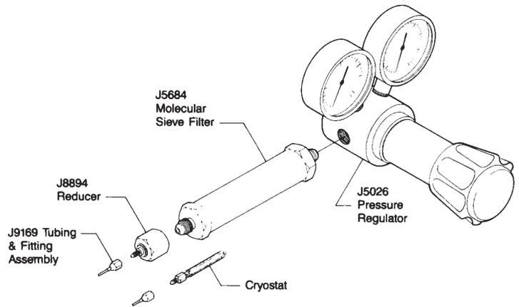
Figure 2: Complete High-Pressure Gas Supply Assembly for Joule-Thomson Cryostat Operation
