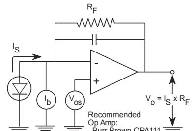
Max.  $R_F$  for InSb determined by  $(I_{BG})$  Fig. 19-5.
