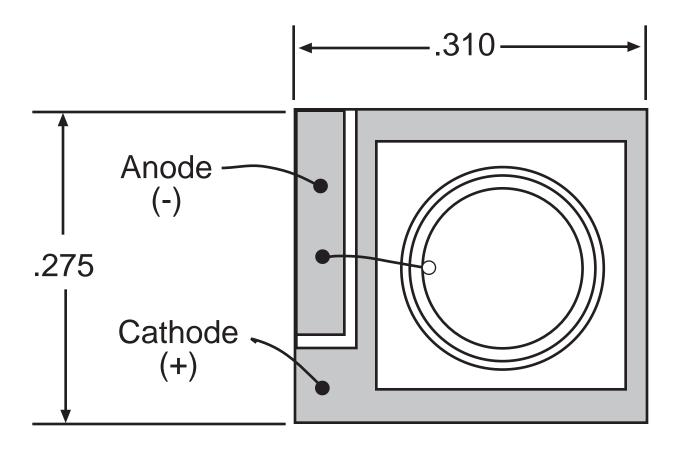
Note: .010 thick ceramic substrate used for both C11 and C12.
