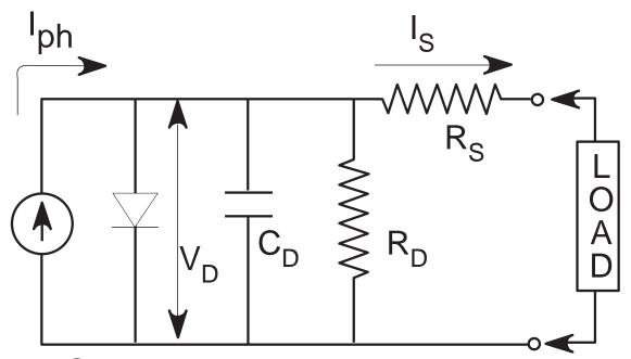
I<sub>ph</sub> = Current generated by incident photonsV<sub>D</sub> = Actual voltage across diode junction
