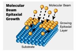
the material layer-by-layer in a regulated process under pure and controlled conditions, resulting in a superior final product.
